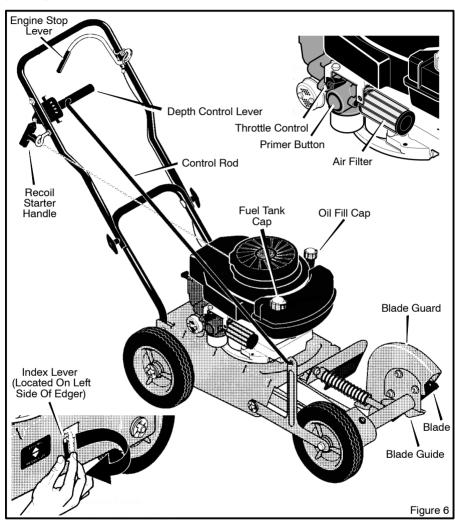
**Throttle Control** – The engine is set to run at full speed. The throttle control has only two positions, RUN and STOP.
